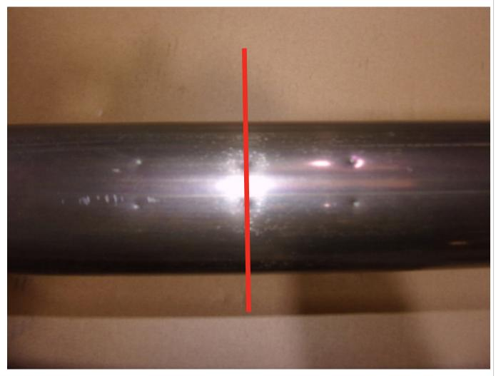
To make it easier to cut the exhaust we reccomend remoiving it from the car. Find the 3 pairs of indents and use the middle pair to mark out the cutting line. Cut along the line and de-bur the edges. Fit the Scorpion GPF delete and fit the original GPF-back or the Scorpion GPF-back system.
